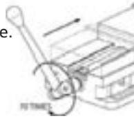
Cap screws need to be removed to change jaws. No way to accurately relocate.
