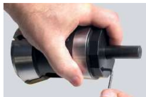
Lock stopper housing in position
