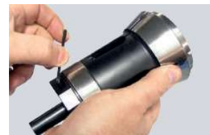
Lock stopper shaft and install
