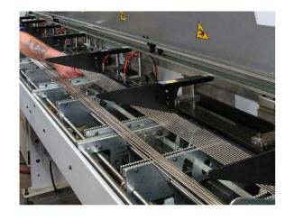
For feeding bar less than 12 mm in diameter, a magazine like the lemca Elite 220 is often preferred, as it has the ability to be swapped quickly from gravity feed of larger bar to walkingbeam advancement of small stock down to 2 mm diameter. The unit features a bar pusher with dual bearings to complement the high performance of Swiss-type machines, with their rapid acceleration and high rotational speeds.
