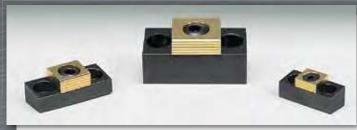
This cam action fixture clamp provides positive down force while using very little space on a fixture. Workpieces can be clamped in series by using the back surface of a clamp to locate the next workpiece. The hardened steel clamping element has both a smooth surface for machined workpieces and a serrated clamping surface for rougher work. The height of the clamp can be adjusted by milling the slot deeper in the fixture plate.
