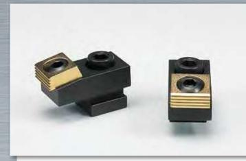
This clamp is like the Compact Toe Clamp, only it is designed to be used in the T-slots of machine tables. It provides 4,000 lbs. (17800 N) positive down force while maintaining a low profile. The hardened steel clamping element has both a smooth surface for machined workpieces and a serrated clamping surface for rougher work.
