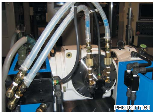
● Installation of optional rotary joint
