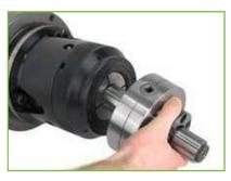
Load the KEM-MA manual actuator into a three jaw or collet chuck, gripping on the 38mm location spigot.
