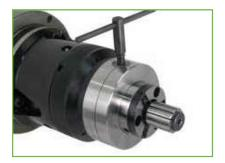
Load a workpiece's internal diameter over the sleeve and actuate the mandrel using the key provided.
