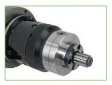
Actuate the power chuck to ensure KEM-MA is locked in position, adjust T.I.R as required.
