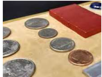
The original paper product is excellent for holding smooth flat parts and maintaining parallelism.
