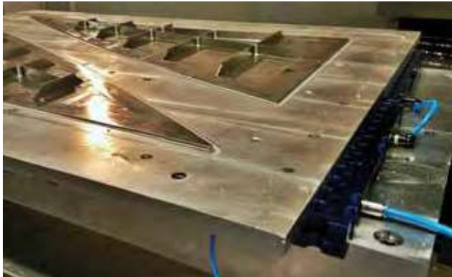
Multiple MPV's shown with large vacuum pallet.
