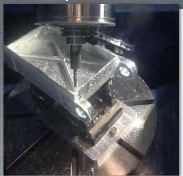
The Loc-Jaw® system was conceived to simplify, and allow greater tooling access and more versatility securing your parts when 4th and 5th axis machining. Designed to hold raw stock without a pre-op using the carrier method. New Combo Edge Grippers incorporate both Knife and Blunt-Edges in one grip.
