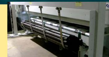
The Master Verso is available also in the version 100. This model is able to load bars up to 102 mm. The new bundle magazine doesn't require the use of the overhead crane to be loaded.
