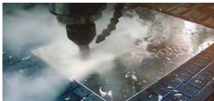
Application using Mitee-Grip™ with sacrificial top plate
