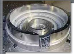
The popular Pitbull® Fixture Clamp is now available in a machinable version. The clamp has positive down force and a very low gripping profile, reducing material cost and number of operations.
