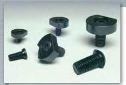
These clamps, with the machinable steel washers, provide more flexibility for holding round or unusual shaped parts. Parts can be held directly to the fixture plate surface or elevated for through drilling. A special screw is provided with each package to hold the washer in the proper place during machining.
