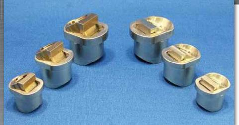
The majority of the Dyna-Force® clamp is below the surface of the fixture which provides excellent clamp support and makes for a very low profile. The clamp jaw slides on an angle for positive downforce.
