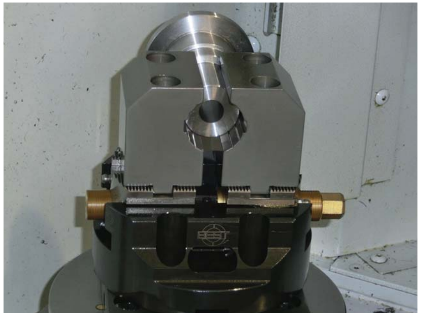
BSM-140 with mould jaws (customer-specific) for the clamping of a turning piece with 35 mm diameter.
