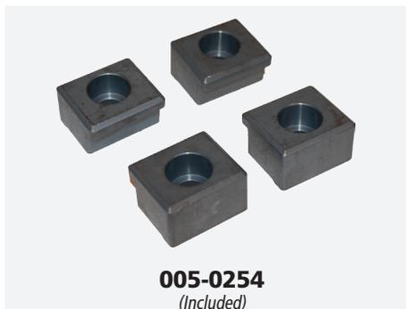
Toe Clamps (four per set) mount a OneLOK to a T-slotted VMC table. Toe Clamps can be used with either a 1/2-13 or M12 socket-headed cap screw. (T-nuts and cap screws not included).
