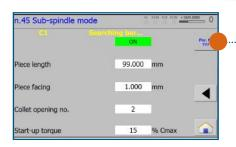
**Sub-spindle software mode** allows higher working speeds and lower unproductive times. Thanks to the measurement of the length of the bar introduced into the spindle, it is able to keep track of the number of finished pieces and to detect when to load a new bar, only requiring the operator to initially insert a few parameters.
