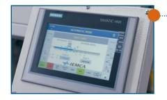
The **new one touch operator interface** can facilitate usage by less experienced operators and also has the ability to **store part programs** (up to 100) and easily recall them when needed by the operator. It is possible to remotely operate the bar feeder from the panel of the lathe\*\*\*.
