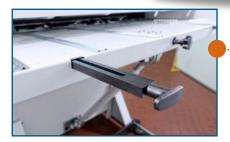
The **simplified bar loading kit** allows simpler and safer loading of heavy bars into the magazine.
