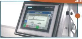
The **new "one touch" operator interface** facilitates usage by less experienced operators and also has the ability to memorize work programs and easily recall them if needed. It is possible to remotely operate the barfeeder from the panel of the lathe\*
