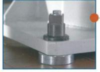
The coaxial fastening system fixed to the floor ensures **stability** of the barfeeder
