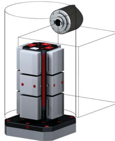
Workholding package in machine envelope
