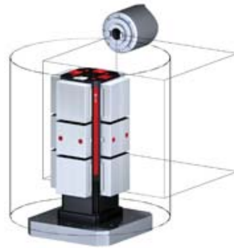
Workholding package in machine envelope
