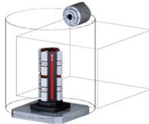
Workholding package in machine envelope
