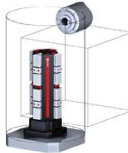
Workholding package in machine envelope
