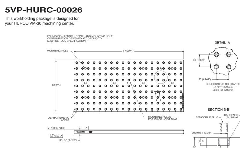
FOUNDATION MAT'L: CAST IRON FOUNDATION INCLUDES INSTALLATION HARDWARE
