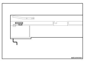
• Bring the first feeding carriage to its backward stroke limit and insert the bar pusher.
