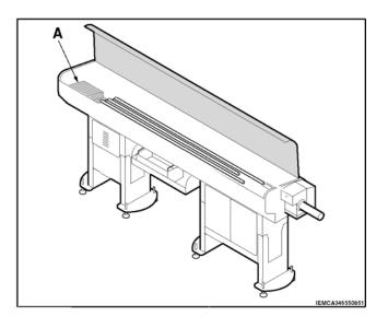
The oil flow in the guide channels and bush holder device is automatically controlled during the bar feeder automatic cycle.
