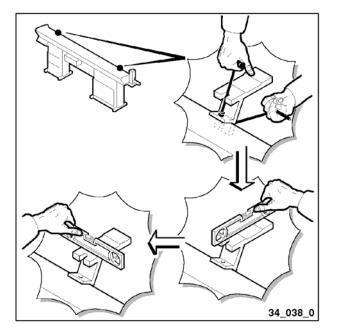
• Carry out the required corrections by turning the support feet screws.
