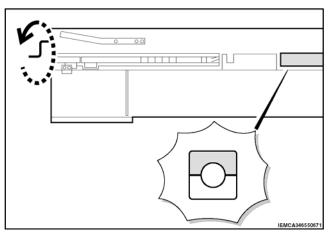
• Move the bar pusher forwards and backwards in the flag area to make sure that its stroke is not hindered.
