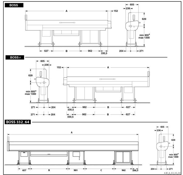
(\*) Without axial displacement device, the minimum value can be decreased to 850 mm.
