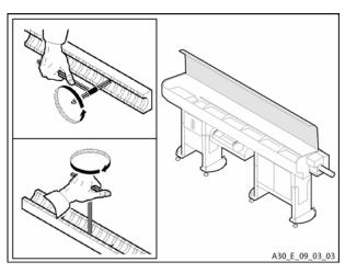
Assemble the "snap in" pins.
