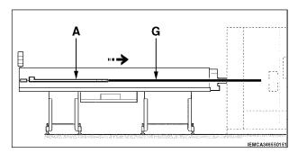
The clamps "D" close, the bar pusher "A" moves forwards; the bar "G" is inserted into the bar
