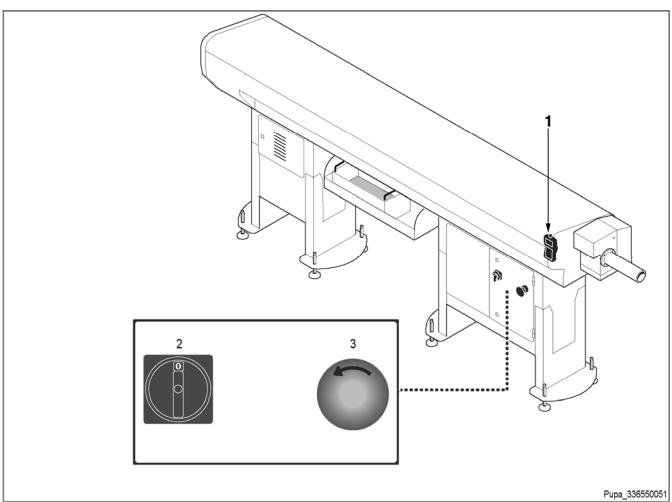
The figure indicates the positions of both the electrical and handheld keyboard "1" controls.
