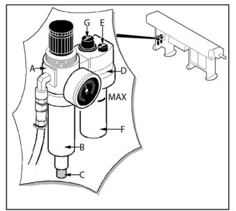
• Restore the compressed air supply. Check air lubrication (1-12 drops every 1,000 l. of air), adjust by turning the screw "G".
