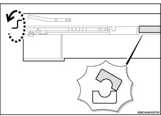
Manually lift the lower lever and replace the clamp. Remove the intermediate gate if necessary (see "GUIDE CHANNELS, HALF BUSHES, BAR PUSHER AND COLLET -REPLACEMENT", CH. 5).
