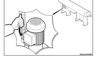
• Adjust oil flow in the bush holder device as well.
