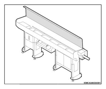
• Close the upper guide channels (sensor "A" must be energized).
