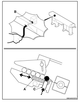
• Open the upper guide channels; the first bar must be dropped into the guide channels, while the second bar should be held in the magazine until the next guide channel closure.
