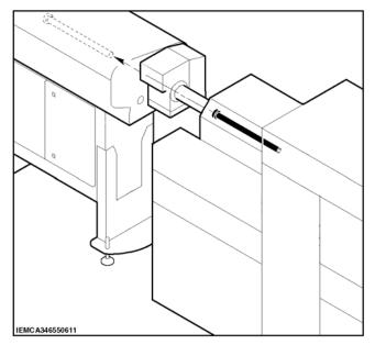
Install front half bushes suitable for the bar in the following way:
