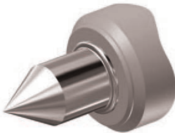
Full-diameter long point for shaft work and parts with large center holes.
