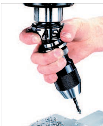
3. Removing drill chuck holder with one hand.
