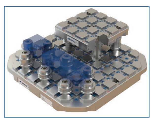
**Example:** Cylindrical supports being used to provide additional support to a workpiece during machining operations. The support helps to center the workpiece and keep it stable, improving accuracy and precision. The cylindrical shape of the support makes it ideal for use with round or cylindrical workpieces. This support is commonly used in conjunction with other clamping devices to ensure optimal machining results. These supports also work as risers for pallets or workpieces.
