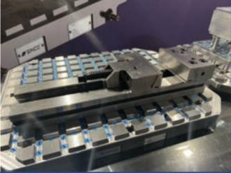
**Real-life example:** The rails are placed underneath the clamping equipment and provide precise positioning, ensuring that the workpiece is held securely in place. By retrofitting existing clamping equipment, machinists can save time and money while still achieving the benefits of the MultiZero system, including quick and easy adjustments and reliable stability during machining operations.
