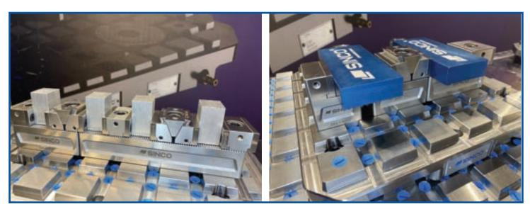
**Real-life example:** By using the MultiZero Vise Double Wedge in conjunction with the MultiZero Clamping System, machinists can achieve efficient and precise production with minimal effort. The modular design of the vise also allows for easy customization and integration with other MultiZero components.
