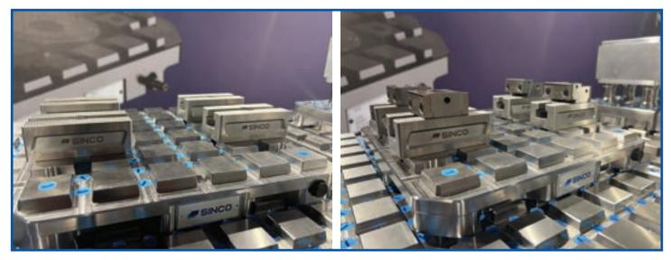
**Real-life example:** The system is highly modular, allowing for easy customization and integration with other MultiZero components. The rails provide a secure foundation for the vise, ensuring reliable stability and precise positioning during machining operations. By using the MultiZero Vise system in conjunction with the MultiZero Clamping System, machinists can achieve optimal results with minimal effort.
