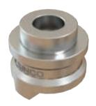
■ Cylindrical support with two support heights, 35 and 25 mm; tightened with M12 screw from the top; positioning rib on the underside
