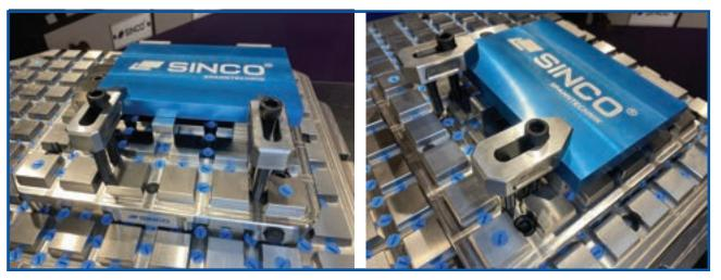
**Real-life example:** They are easy to adjust and can be used with a variety of workpiece sizes and shapes. By using MultiZero Clamps with the MultiZero system, machinists can achieve reliable stability and precise positioning of the workpiece, resulting in optimal machining results.
